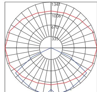
Maximum Candela = 1340.9 Located At Horizontal Angle = 0, Vertical Angle = 5
