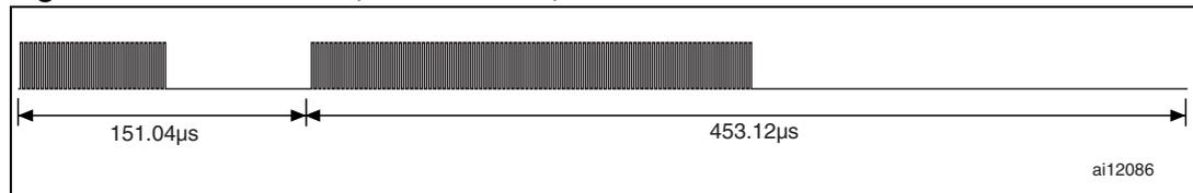
For the Fast commands, the EOF comprises a logic 0 that includes 16 pulses at 423.75 kHz and an unmodulated time of 37.76  $\mu\text{s}$ , followed by 48 pulses at 423.75 kHz ( $f_C/32$ ) and an unmodulated time of 113.28  $\mu\text{s}$  as shown in [Figure 33](#).
