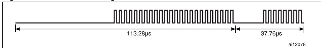
For the Fast commands, the SOF comprises an unmodulated time of 28.32  $\mu\text{s}$ , followed by 12 pulses at 423.75 kHz ( $f_C/32$ ), and a logic 1 that consists of an unmodulated time of 9.44  $\mu\text{s}$  followed by 4 pulses at 423.75 kHz as shown in [Figure 25](#).
