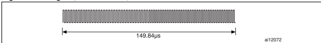
A logic 1 starts with 36 pulses at 484.28 kHz ( $f_C/28$ ) followed by 32 pulses at 423.75 kHz ( $f_C/32$ ) as shown in [Figure 23](#). For the Fast commands, the x2 mode is not available.
