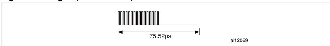
A logic 1 starts with an unmodulated time of 75.52  $\mu\text{s}$  followed by 32 pulses at 423.75 kHz ( $f_C/32$ ) as shown in [Figure 18](#).
