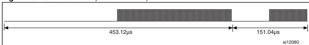
For the Fast commands, the SOF comprises an unmodulated time of 113.28  $\mu\text{s}$ , followed by 48 pulses at 423.75 kHz ( $f_{\text{C}}/32$ ), and a logic 1 that includes an unmodulated time of 37.76  $\mu\text{s}$  followed by 16 pulses at 423.75 kHz as shown in [Figure 27](#).
