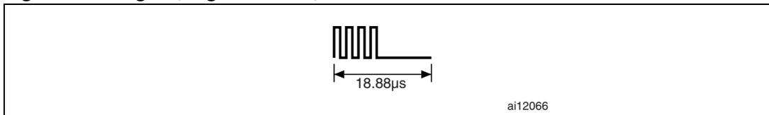
A logic 1 starts with an unmodulated time of 18.88  $\mu s$  followed by 8 pulses at 423.75 kHz ( $f_C/32$ ) as shown in [Figure 14](#).
