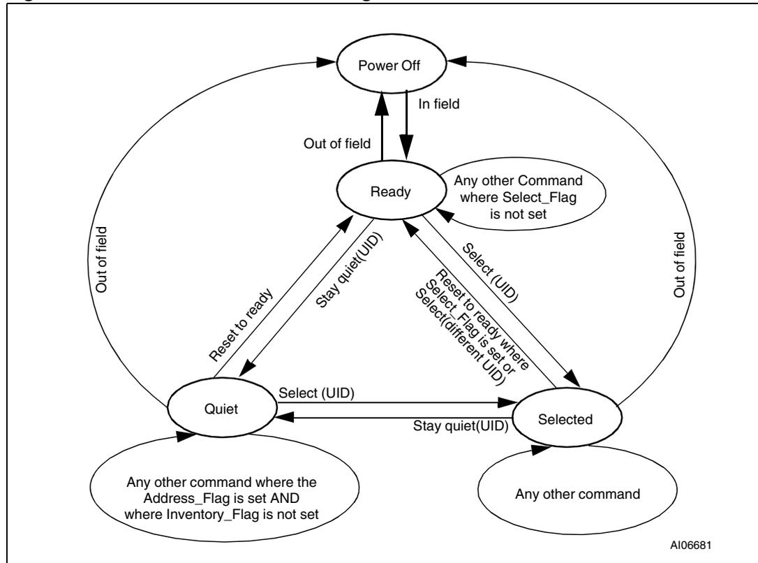
1. The intention of the state transition method is that only one LRIS64K should be in the selected state at a time.
