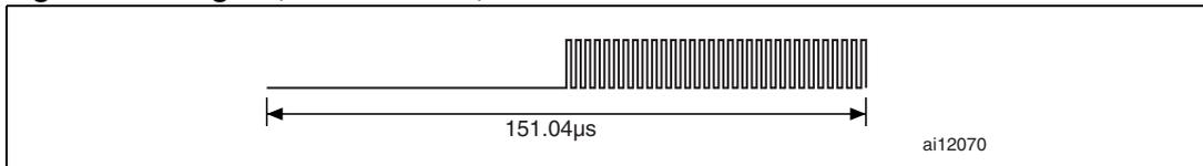
For the Fast commands, a logic 1 starts with an unmodulated time of 37.76  $\mu\text{s}$  followed by 16 pulses at 423.75 kHz ( $f_C/32$ ) as shown in [Figure 18](#).
