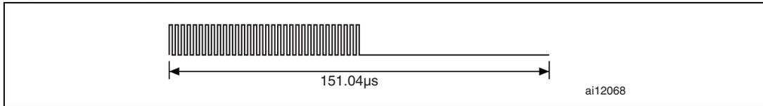
For the Fast commands, a logic 0 starts with 16 pulses at 423.75 kHz ( $f_C/32$ ) followed by an unmodulated time of 37.76  $\mu\text{s}$  as shown in [Figure 17](#).
