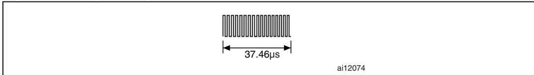
A logic 1 starts with 9 pulses at 484.28 kHz ( $f_C/28$ ) followed by 8 pulses at 423.75 kHz ( $f_C/32$ ) as shown in [Figure 21](#). For the Fast commands, the x2 mode is not available.
