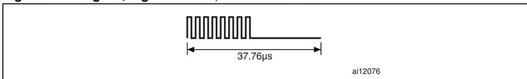
For the fast commands, a logic 0 starts with 4 pulses at 423.75 kHz ( $f_C/32$ ) followed by an unmodulated time of 9.44  $\mu s$  as shown in [Figure 13](#).
