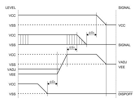
Please maintain the above sequence when turning on and off the power supply of the module. If  $\overline{\text{DISPOFF}}$  is supplied to the module while internal alternate signal for LCD driving (M) is unstable, DC component will be supplied to the LCD panel. This may cause damage the LCD module.
