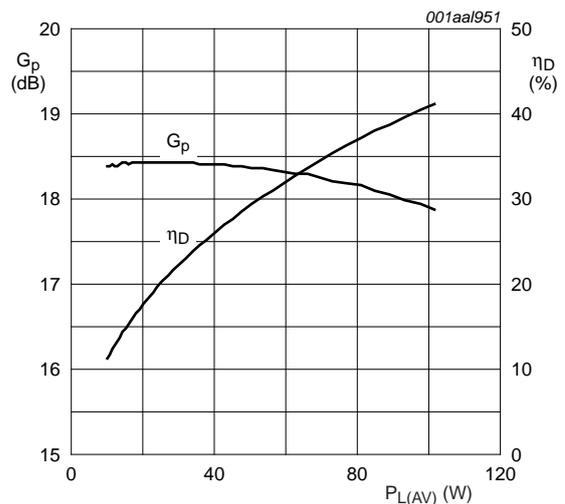
**Fig 5. Power gain and drain efficiency as a function of average output power; typical values**
