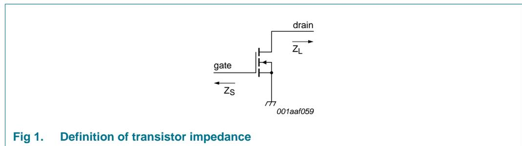
**Fig 1. Definition of transistor impedance**
