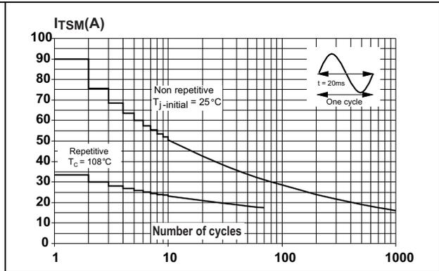
Figure 8. Non repetitive surge peak on-state current for a sinusoidal pulse with width  $t_p < 10$  ms, and corresponding value of  $I^2$
