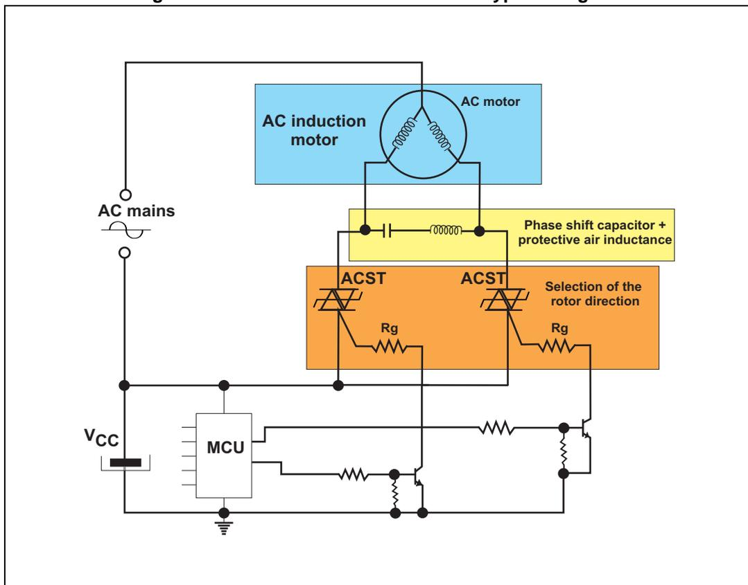
Figure 17. Universal drum motor control – typical diagram
