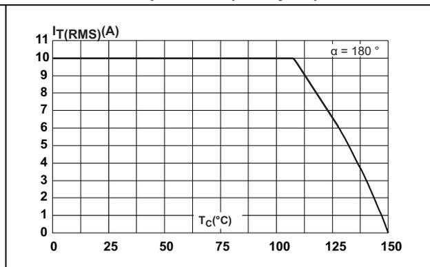
Figure 4. On-state rms current versus ambient temperature (free air convection)
