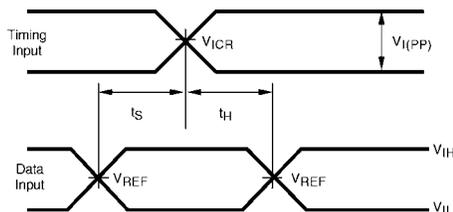
FIGURE 5. Voltage Waveforms - Setup and Hold Times
