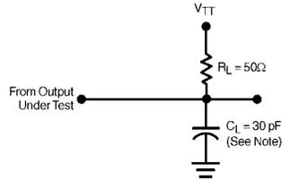
Note:  $C_L$  includes probe and jog capacitance
