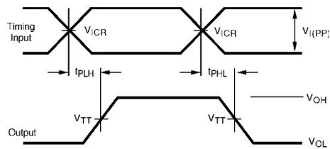
FIGURE 4. Voltage Waveforms - Propagation Delay Times
