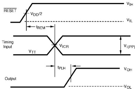
FIGURE 7. Voltage Waveforms - RESET Removal Delay Times
