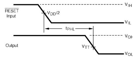
FIGURE 6. Voltage Waveforms - RESET Propagation Delay Times
