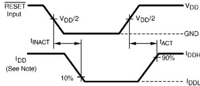
Note:  $I_{DD}$  tested with clock and data inputs held at  $V_{DD}$  or GND, and  $I_O = 0 \text{ mA}$ .
