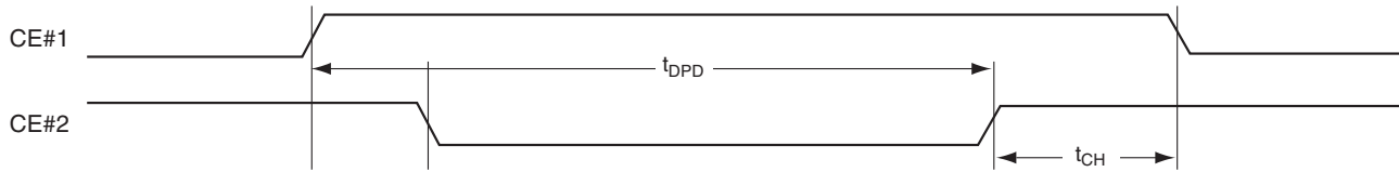
Figure 33. Deep Power-down Timing
