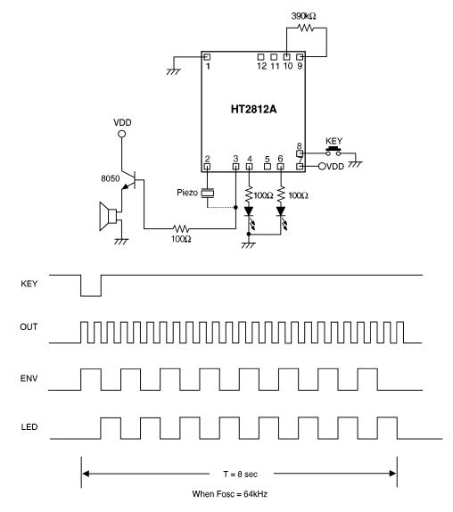
\* The IC substrate should be connected to VDD in the PCB layout artwork.
