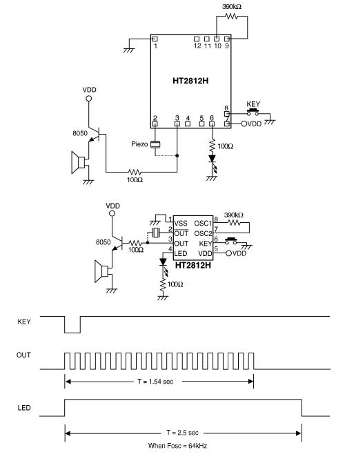
\* The IC substrate should be connected to VDD in the PCB layout artwork.
