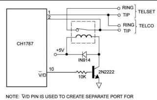
NOTE: \$\tilde{V}\$/D PIN IS USED TO CREATE SEPARATE PORT FOR TELEPHONE CONNECTION SHARING THE TELCO TIP AND RING. \$\tilde{V}\$/D IS TTL COMPATIBLE (I OL=1.6MA, V OL=0.4V) AND IS ACTIVE DURING THE DATA CONNECTION WHICH ISOLATES THE TELEPHONE FROM THE TELCO. (THE RELAY CHOSEN MUST MEET THE APPROPRIATE REGULATORY AGENCY).
