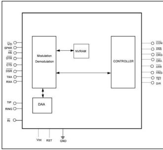
Figure 1. CH1787 Functional Block Diagram.
