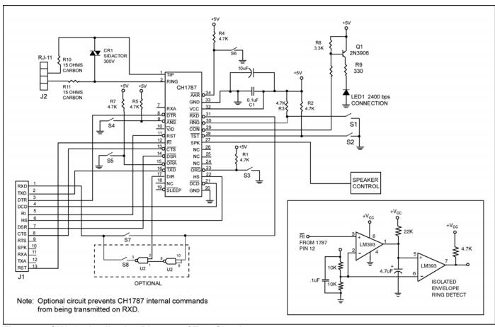
Figure 4. CH1787 Application Diagram of Test Circuit.
