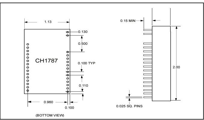
Figure 7. CH1787 Physical Dimensions and Pin Functions.
