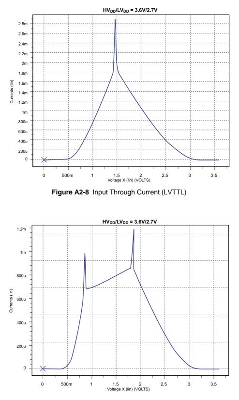
Figure A2-9 Input Through Current (LVTTL Schmitt)
