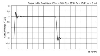
Figure A2-109 Output Waveform (XFLOB3AT)
