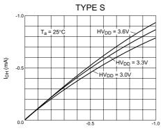
Output voltage  $V_{\text{OH}}$  - Supply voltage  $HV_{\text{DD}}$  (V)
