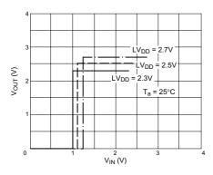
Figure A2-46 Input Characteristics (CMOS)
