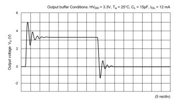
Figure A2-43 Output Waveform (XFHOB3AT)
