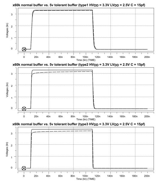
Figure A2-124 Comparison between 5 V Tolerant Fail-Safe Cells and Normal Cells
