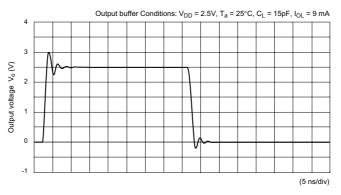
Figure A1-77 Output Waveform (XOB3T)
