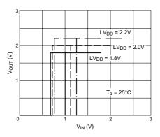
Figure A2-80 Input Characteristics (CMOS Schmitt)
