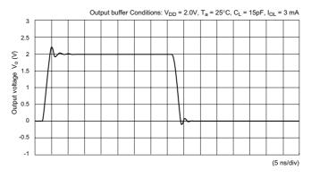
Figure A1-110 Output Waveform (XOB3T)
