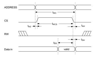
Figure 6-4 Write Cycle (CS Control)
