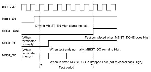
Figure 10-12 Test Sequence of the Memory BIST Circuit
