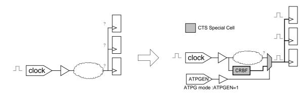
Figure 10-18 Processing of Internally Generated Clocks
