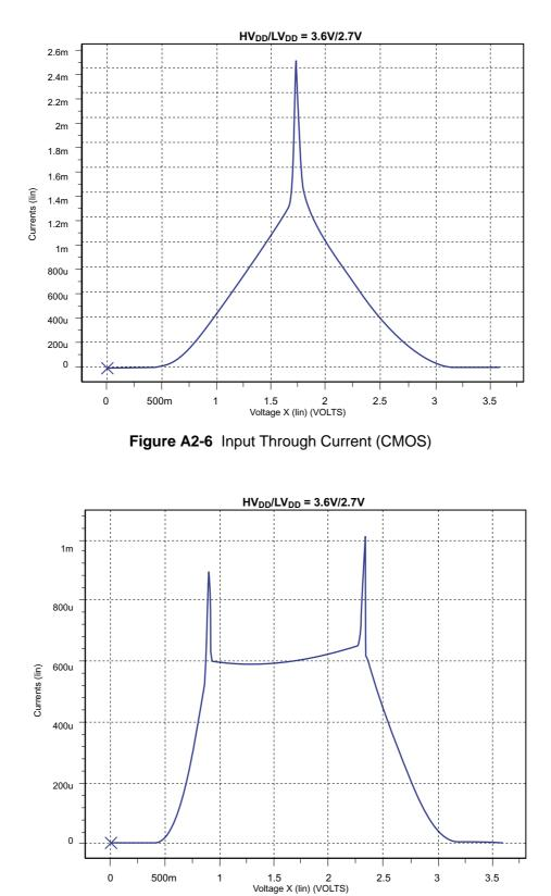
Figure A2-7 Input Through Current (CMOS Schmitt)
