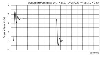
Figure A2-76 Output Waveform (XFLOB3AT)
