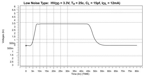
Figure A2-128 Output Waveform (XFHOBF3BT)
