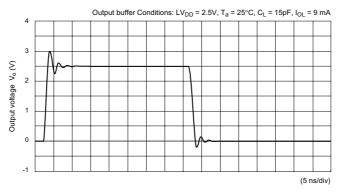
Figure A2-77 Output Waveform (XFLOB3T)
