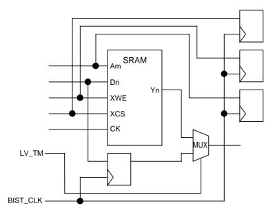
Figure 10-11 Bypass Circuit
