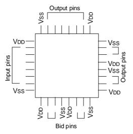
Figure 9-16 Example of Separating Input and Output Pins
