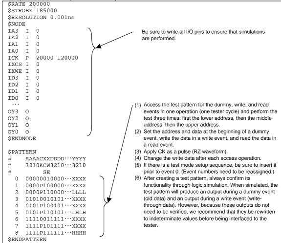
Figure 10-6 Procedure for Creating Test Patterns for 1 port RAM (Synchronous) Test Pattern
