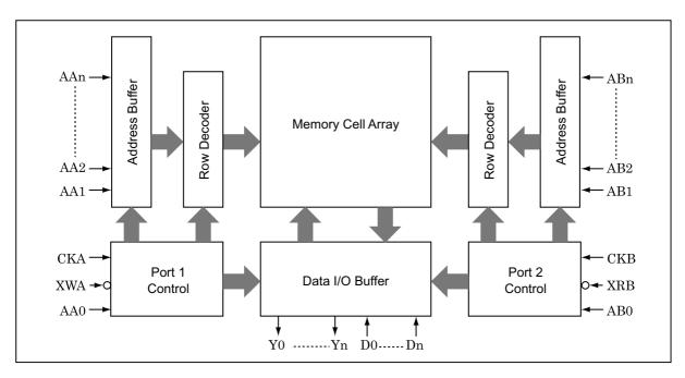
Figure 6-9 Block Diagram of a 2 port RAM (Clock Synchronous Type)
