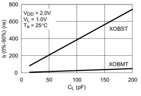
Rising Time (t<sub>r</sub>) vs. Output Load Capacitance (C<sub>L</sub>)
