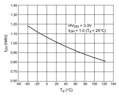
Figure A1-26 Ambient Temperature (T<sub>a</sub>) - Output Current (I<sub>OH</sub>)
