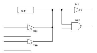
Figure 9-7 Typical Configuration of a Bus Cell Circuit
