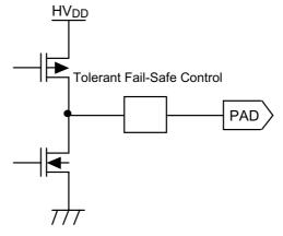
Figure A2-112 Output Buffer Structure of 5 V Tolerant Fail-Safe Cell
