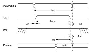
Figure 6-7 Write Cycle (CS Control)
