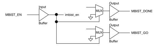
Figure 10-14 Image of a Circuit Description
