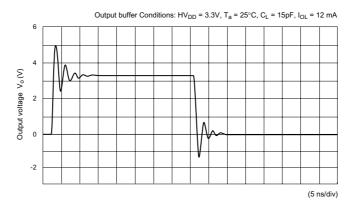
Figure A1-43 Output Waveform (XHOB3AT)
