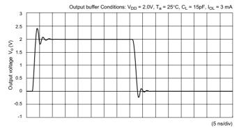
Figure A1-109 Output Waveform (XOB3AT)
