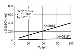
Output buffer rising/falling time vs. Output load capacitance (CL)
