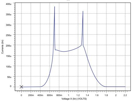
Figure A2-82 Input Through Current (CMOS Schmitt)
