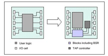
Figure 10-24 Image of a Hierarchical Block Configuration
