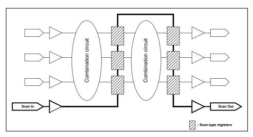
Figure 10-15 Example of a Scan Circuit
