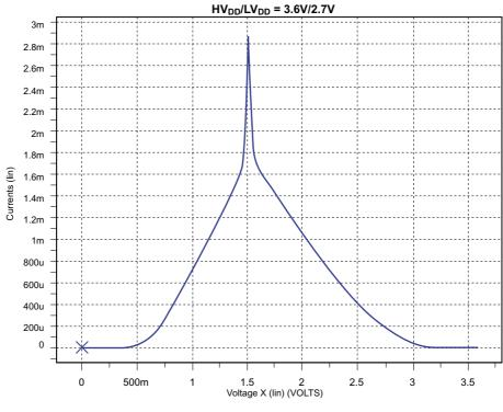
Figure A2-10 Input Through Current (PCI)
