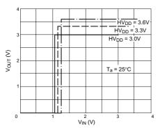
Figure A2-3 Input Characteristics (PCI-3V)
