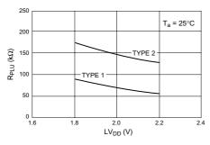
**Figure A2-105** Pull-up Resistance (R<sub>PLU</sub>) vs. LV<sub>DD</sub>
