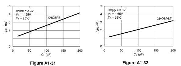
Output Delay Time (t<sub>pLH</sub>) vs. Output Load Capacitance (C<sub>L</sub>) Output Delay Time (t<sub>pHL</sub>) vs. Output Load Capacitance (C<sub>L</sub>)
