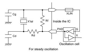
Figure 9-11 Crystal Oscillation Circuit (I/O Cell Type)
