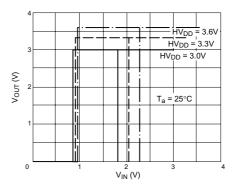
Figure A2-5 Input Characteristics (CMOS Schmitt)
