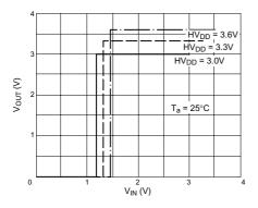
Figure A1-1 Input Characteristics (LVTTL)
