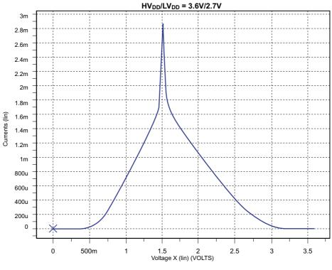
Figure A1-10 Input Through Current (PCI)
