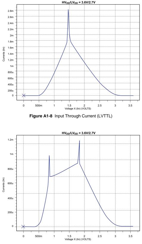
Figure A1-9 Input Through Current (LVTTL Schmitt)
