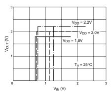
Figure A1-80 Input Characteristics (CMOS Schmitt)
