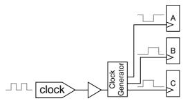
Figure 10-20 (a) Example with Multiple Internally Generated Clocks
