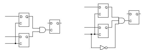
Figure 9-9 Example of Hazard Protection
