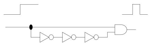
Figure 9-4 Example of a Bad Differentiating Circuit
