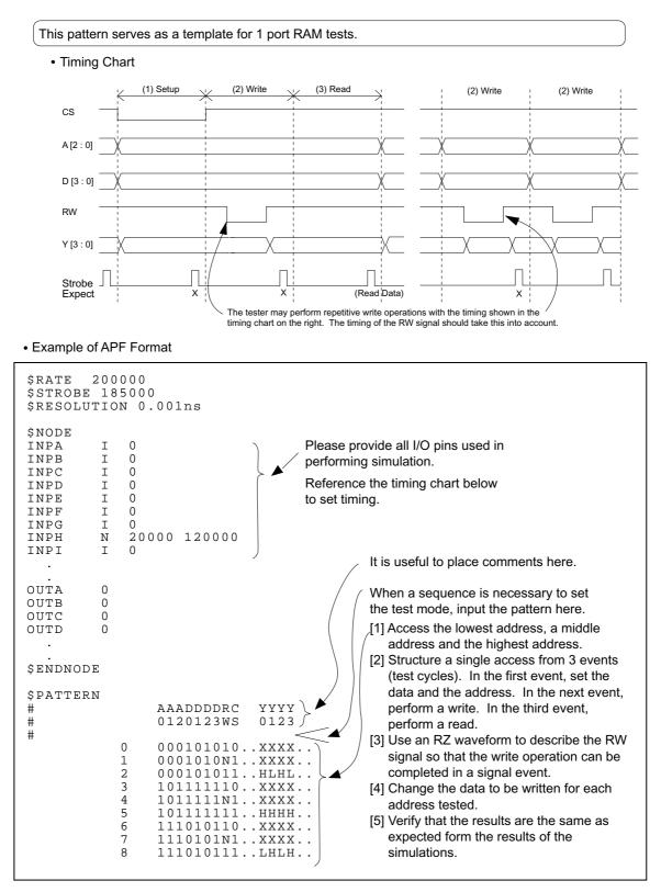
Figure 10-4 Generating 1 port RAM Test Pattern
