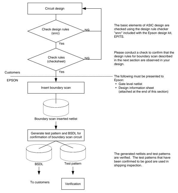
Figure 10-22 Boundary Scan Design Flow
