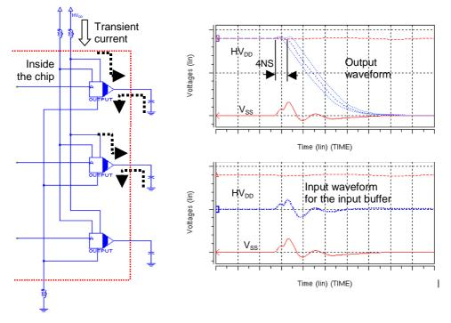
Figure 9-13 Noise due to Simultaneous Operation of Outputs
