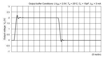
Figure A2-110 Output Waveform (XFLOB3T)
