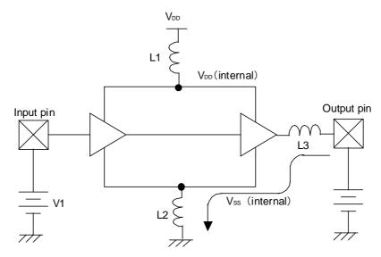
Figure 9-15 LSI Equivalent Circuit
