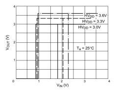
Figure A1-5 Input Characteristics (CMOS Schmitt)
