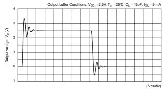
Figure A1-76 Output Waveform (XOB3AT)
