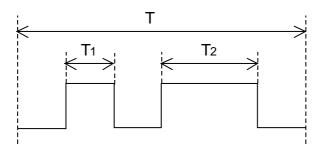
Figure 8-3 Example of a Duty Cycle
