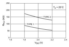
**Figure A1-105** Pull-up Resistance (R<sub>PLU</sub>) vs. V<sub>DD</sub>
