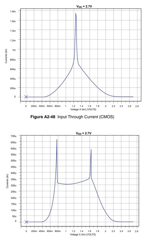
Figure A2-49 Input Through Current (CMOS Schmitt)
