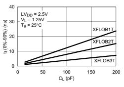
Falling Time (t<sub>f</sub>) vs. Output Load Capacitance (C<sub>L</sub>)
