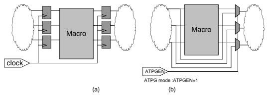
Figure 10-21 Example of Macro Cell Processing
