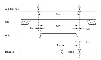
Figure 6-6 Write Cycle (WR Control)
