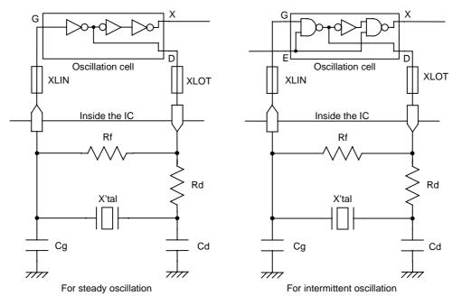
Figure 9-10 Crystal Oscillation Circuit (Internal Cell Type)
