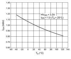
Figure A2-26 Ambient Temperature (T<sub>a</sub>) - Output Current (I<sub>OH</sub>)
