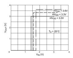
Figure A2-2 Input Characteristics (CMOS)
