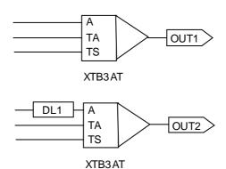
Figure 9-22 Example of Adding Delay Cells
