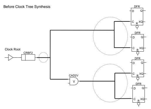
Clock Tree Synthesis optimizes the skew value for the thick-lined parts.
