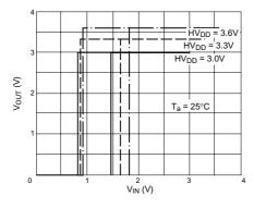
Figure A1-4 Input Characteristics (LVTTL Schmitt)
