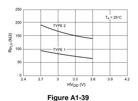
Pull-up Resistance (R<sub>PLU</sub>) vs. HV<sub>DD</sub>
