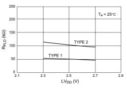
Figure A2-74 Pull-down Resistance (R<sub>PLD</sub>) vs. LV<sub>DD</sub>
