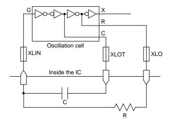
Figure 9-12 CR Oscillation Circuit
