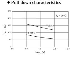
Figure A2-107 Pull-down Resistance ( $R_{PLD}$ ) vs.  $LV_{DD}$
