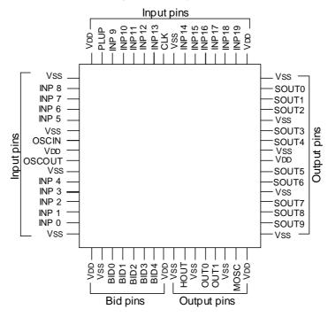
Figure 9-24 Example of the Recommended Pin Layout
