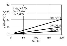
$\label{eq:Figure A2-70} Figure \ A2-70$  Rising Time (t,) vs. Output Load Capacitance (CL)
