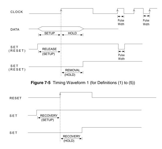
Figure 7-6 Timing Waveform 2 (for Definitions (6) to (7))
