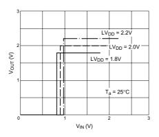
Figure A2-79 Input Characteristics (CMOS)
