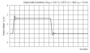
Figure A2-44 Output Waveform (XFHOB3T)
