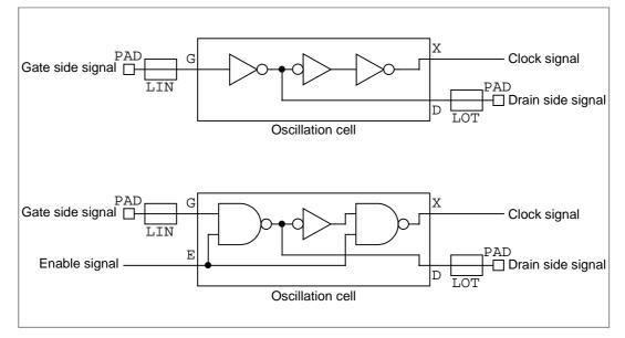
Figure 11-2 Examples of Oscillation Circuits
