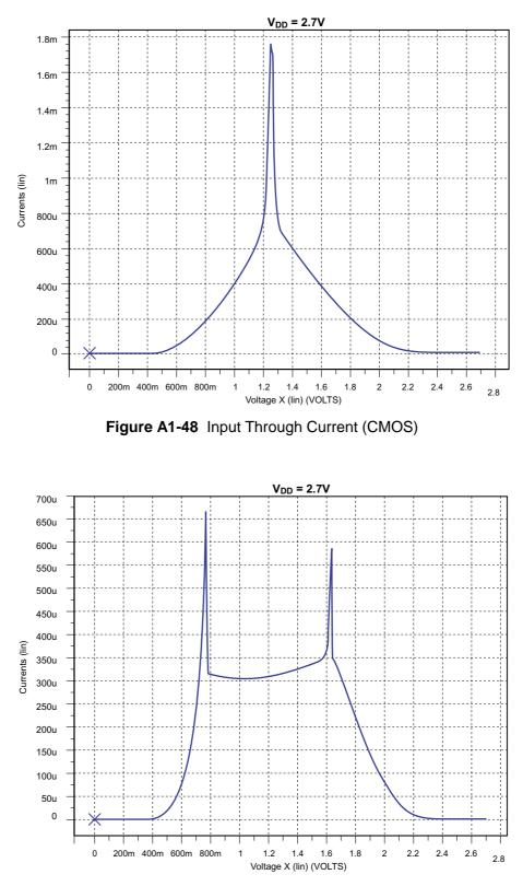
Figure A1-49 Input Through Current (CMOS Schmitt)
