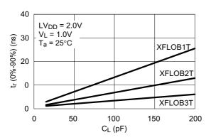
Rising Time  $(t_r)$  vs. Output Load Capacitance  $(C_L)$
