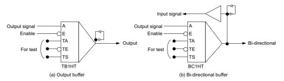
Figure 9-8 Example of a Bus Hold Circuit Symbol
