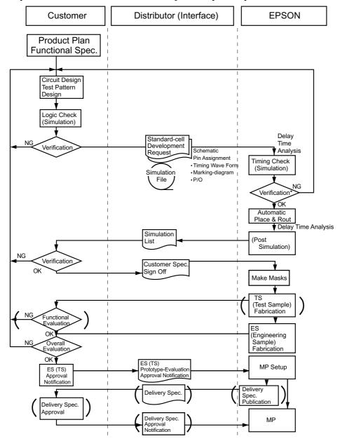
The process flow of the embedded array development process is shown below.
