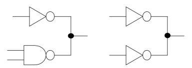
Figure 9-1 Examples of Forbidden Wired Logic
