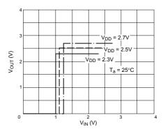
Figure A1-46 Input Characteristics (CMOS)
