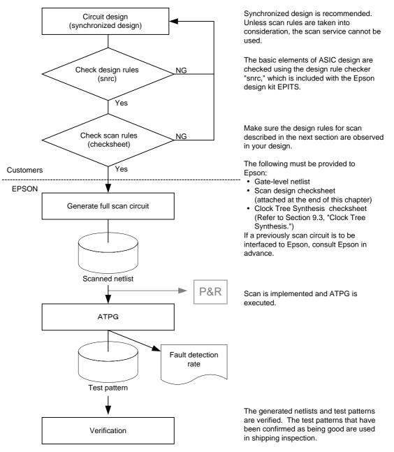
Figure 10-16 Scan Design Flow
