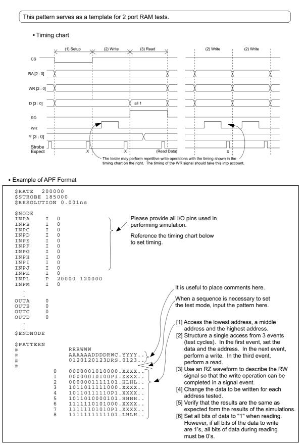
Figure 10-5 Generating 2 port RAM Test Pattern
