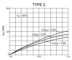
Output voltage  $V_{\text{OH}}$  - Supply voltage  $LV_{\text{DD}}\left(V\right)$
