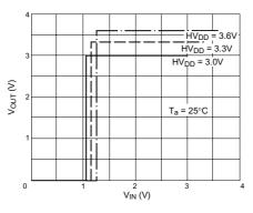
Figure A1-3 Input Characteristics (PCI-3 V)
