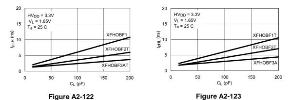
(4) Output delay time vs. Output load capacitance (CL)
