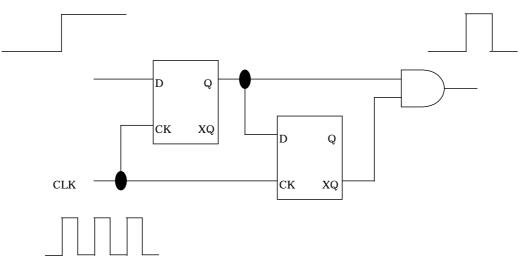
Figure 9-5 Example of a Differentiating Circuit Built with FFs
