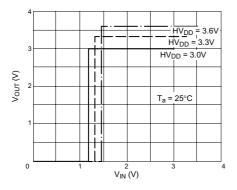
Figure A2-1 Input Characteristics (LVTTL)
