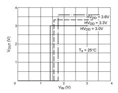
Figure A1-2 Input Characteristics (CMOS)
