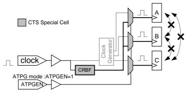
Figure 10-20 (b) Example of a Corrective Measure for Multiple Internally Generated Clocks 1 (When Blocks are Not Interconnected)
