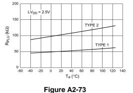
Pull-up Resistance ( $R_{PLU}$ ) vs. Ambient Temperature ( $T_a$ )
