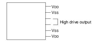
Figure 9-23 Example of Strengthening Power Supplies
