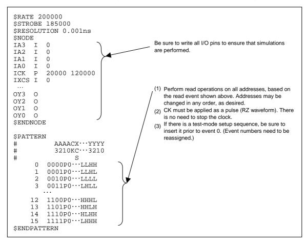
Figure 10-9 Procedure for Creating Mask ROM Tes Patterns
