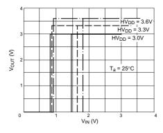
Figure A2-4 Input Characteristics (LVTTL Schmitt)
