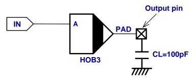
Figure 7-2 Example Circuit for Calculation of the External Cell Propagation Delay Time
