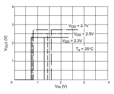
Figure A1-47 Input Characteristics (CMOS Schmitt)
