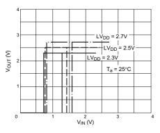
Figure A2-47 Input Characteristics (CMOS Schmitt)
