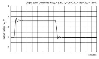
Figure A1-44 Output Waveform (XHOB3T)
