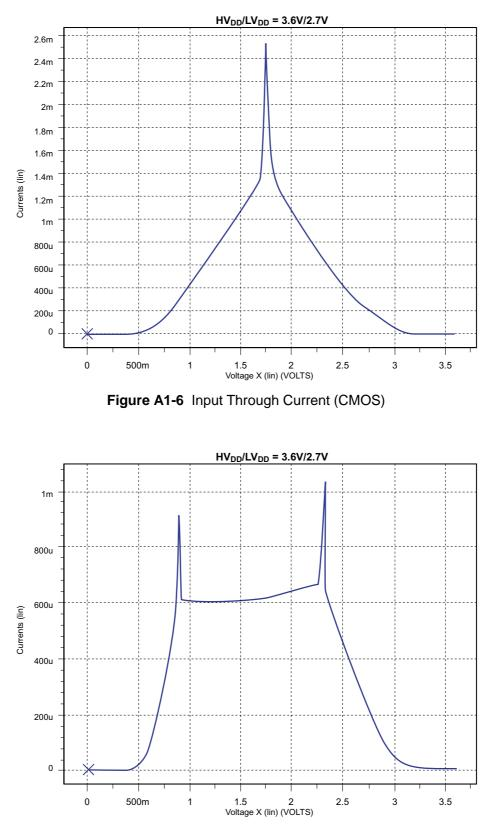
Figure A1-7 Input Through Current (CMOS Schmitt)
