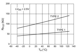
Pull-down Resistance (R<sub>PLD</sub>) vs. Ambient Temperature (T<sub>a</sub>)
