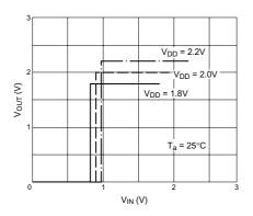
Figure A1-79 Input Characteristics (CMOS)
