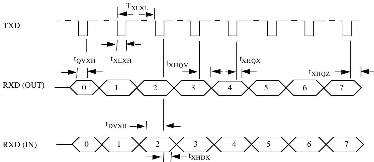
**Figure 12. Serial Port Waveform - Shift Register Mode**
