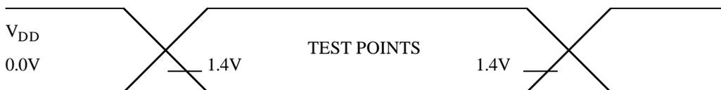
AC Testing inputs are driven at  $V_{DD}$  for a Logic “1” and 0.0V for a Logic “0”. Timing measurements are made at 1.4V.
