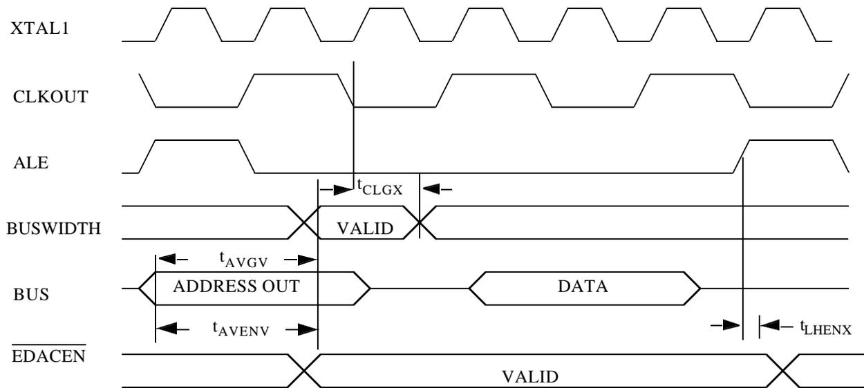
**Figure 6. BUSWIDTH and  $\overline{\text{EDACEN}}$  Timings**
