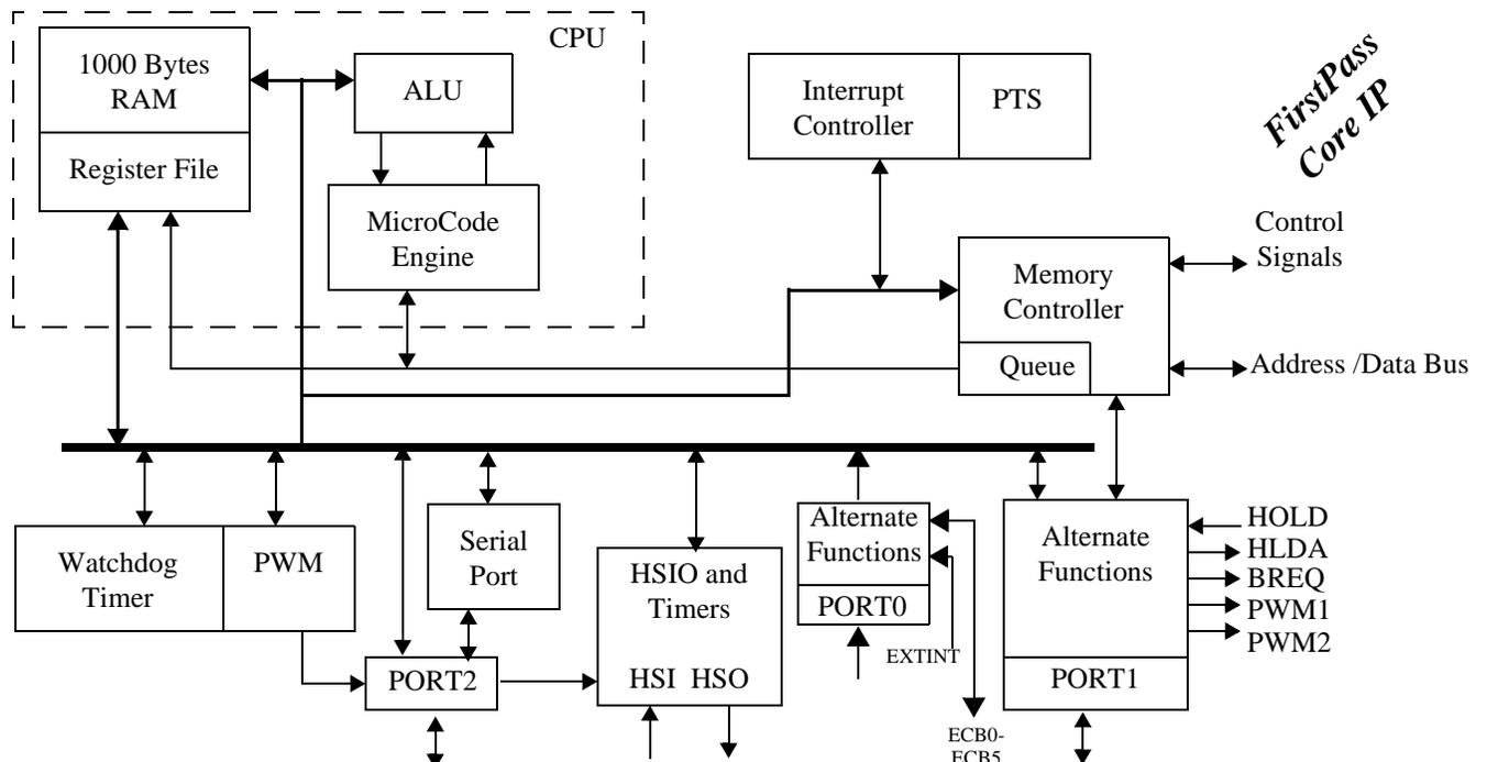
Figure 1. UT80CRH196KDS Microcontroller
