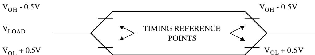
For timing purposes a port pin is no longer floating when it changes to a voltage outside the reference points shown and begins to float when it changes to a voltage inside the reference points shown.  $I_{OL} = 4mA$ ,  $I_{OH} = -4mA$ .
