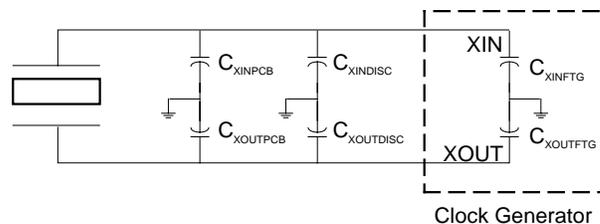
As an example, and using this formula for this datasheet's device, a design that has no discrete loading capacitors (C<sub>DISC</sub>) and each of the crystal to device PCB traces has a capacitance (C<sub>PCB</sub>) to ground of 2pF (typical value) would calculate as:
