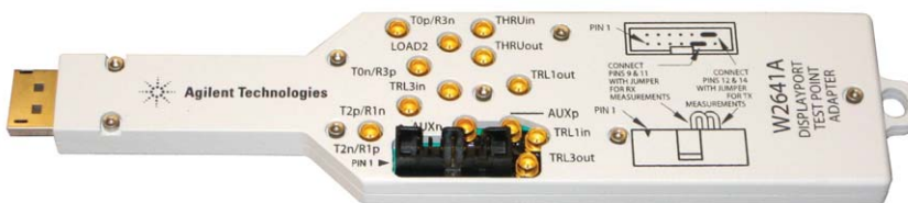
Figure 8: W2641A DisplayPort test point access adaptor.
