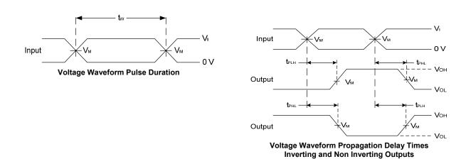
Figure 1. Load Circuit and Voltage Waveforms
