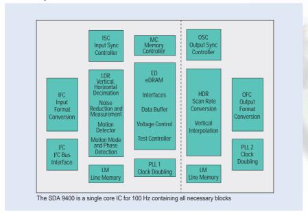
The SDA 9400 contains all necessary functional blocks on a single chip:
