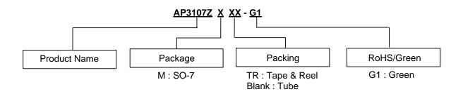
Diodes IC's Pb-free products with "G1" suffix in the part number, are RoHS compliant and green.
