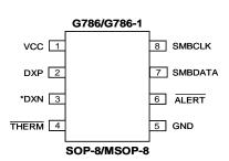
\*: DXN : DXN is internally connected to GND.
