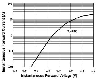
Figure 3. Typical Forward Characteristics Per Diode
