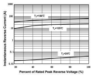
Figure 5. Typical Reverse Characteristics Per Diode
