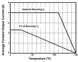
Figure 1. Derating Curve Output Rectified Current
