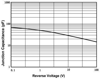
Figure 4. Typical Junction Capacitance Per Diode
