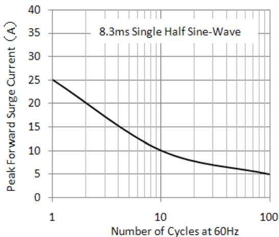
Figure 5. Maximum Non-Repetitive Peak Forward Surge Current
