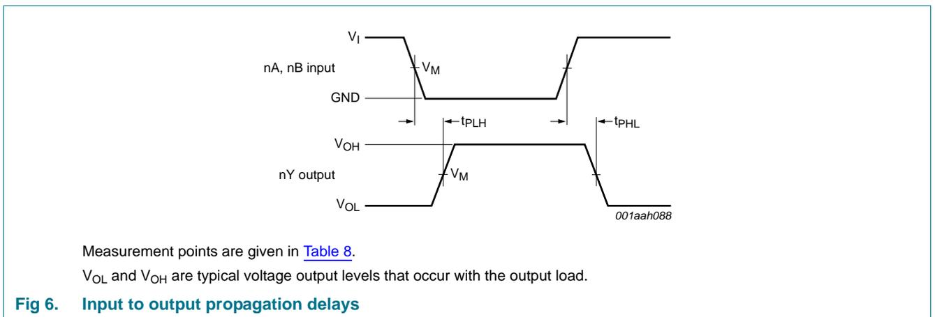
**Fig 6. Input to output propagation delays**
