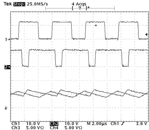
Figure 15 - Inductors current matching.
