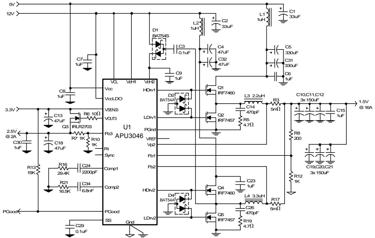
Figure 13 - Demo-board application of APU3046.
