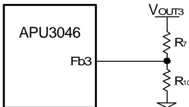
Figure 9 - Programming the output voltage for LDO.
