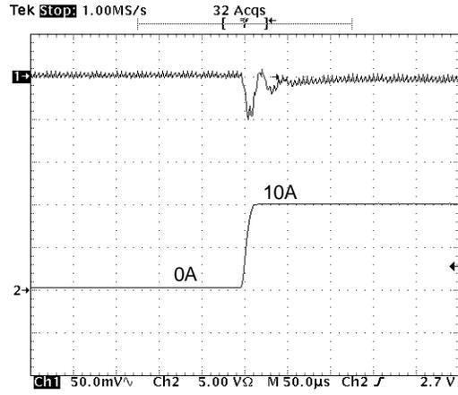
Figure 18 - Transient response @  $I_{OUT} = 0$  to  $10A$ .
