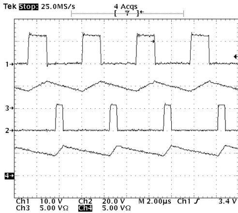
Figure 14 - Gate signals vs. inductor currents.
