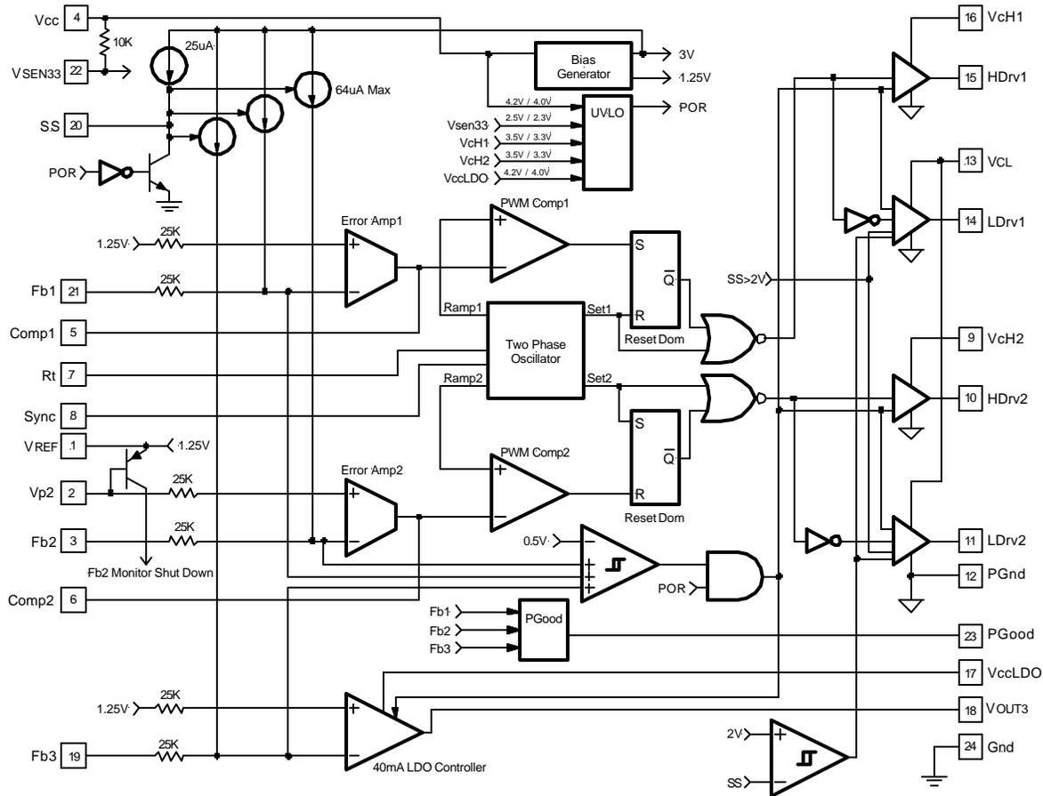
Figure 2 - Block diagram of the APU3046.
