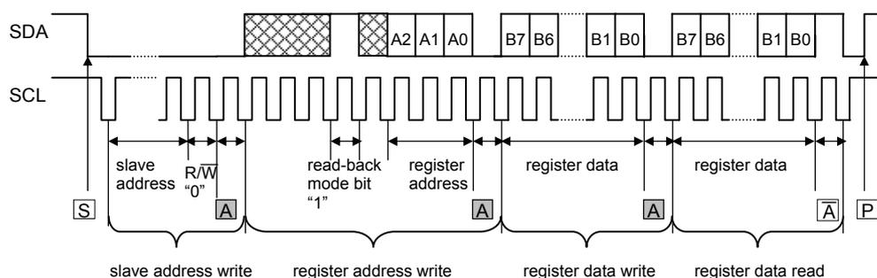
**Figure 5 I<sup>2</sup>C Interface Read Timing: read-back mode**
