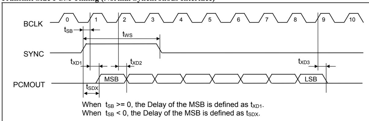
**Transmit Side PCM Timing (Short Frame Synchronous Interface)**
