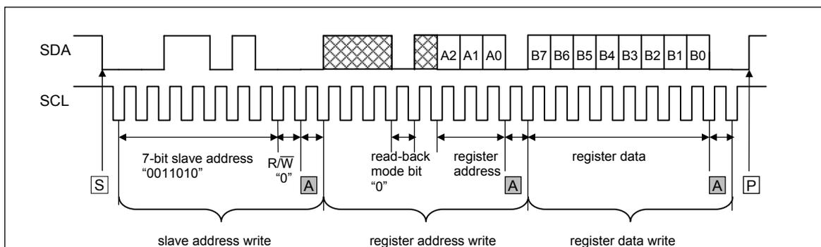
**Figure 3 I<sup>2</sup>C Interface Write Timing**
