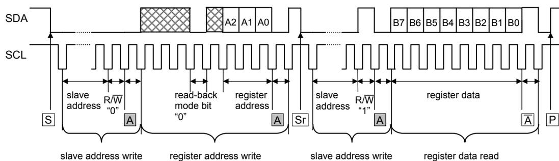
**Figure 4 I<sup>2</sup>C Interface Read Timing: normal mode**
