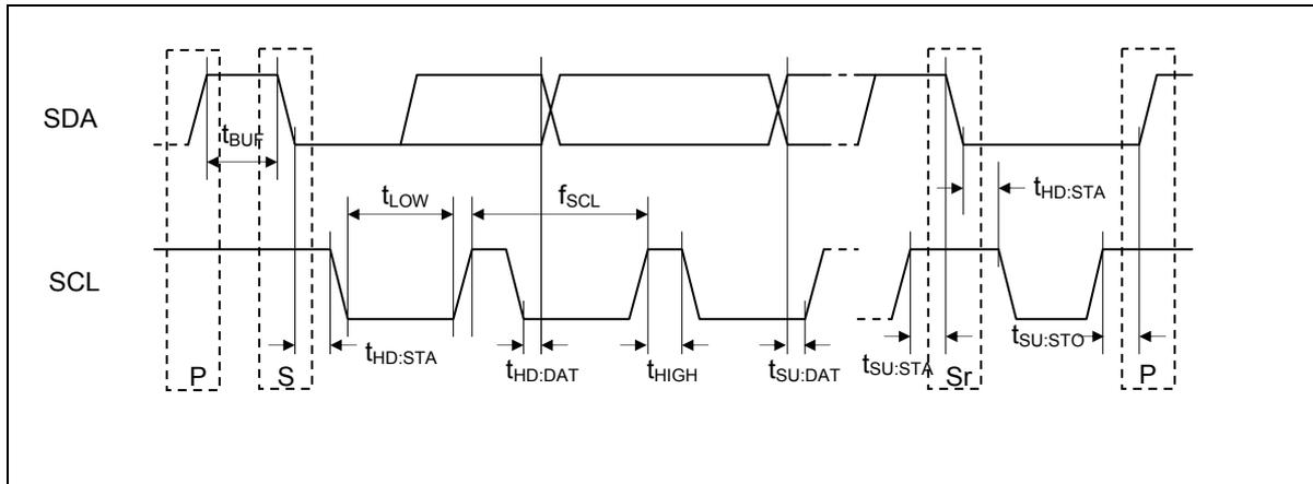
**Figure 7 I<sup>2</sup>C Interface Timing**
