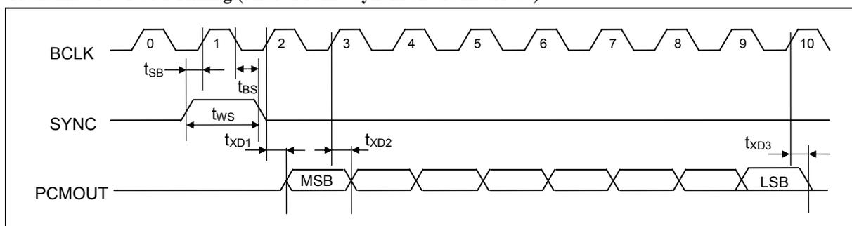
**Receive Side PCM Timing (Normal Synchronous Interface)**
