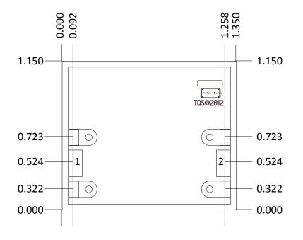
Unit: millimeters Thickness: 0.10Die x, y size tolerance:  $\pm 0.050$ Chip edge to bond pad dimensions are shown to center of pad Ground is backside of die
