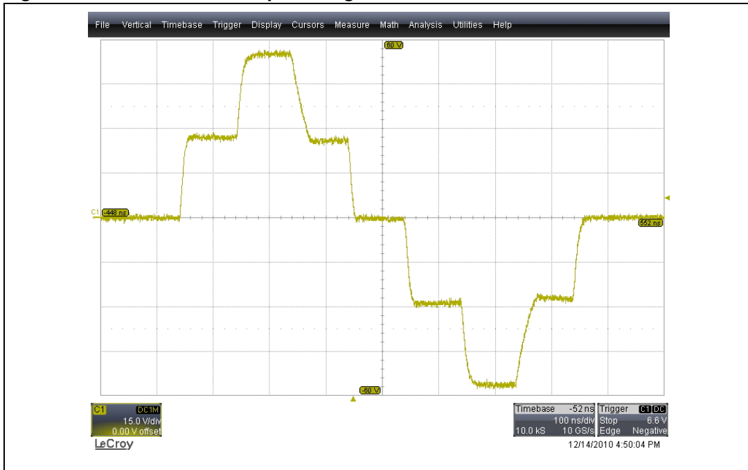
Figure 14. Five-levels HV output voltage
