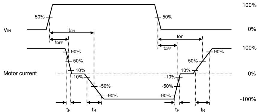
Figure 6. Input-Output AC Characteristic
