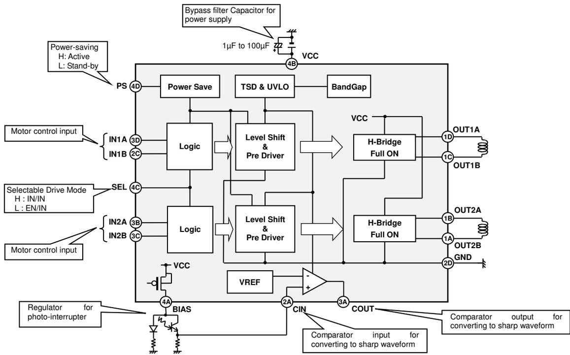
Selection of Components Externally Connected
