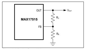
Figure 1. Adjusting Output Voltage
