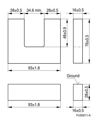
U and I cores are supplied as single units. The  $A_L$  value in the table applies to a core set comprising two ungapped cores.
