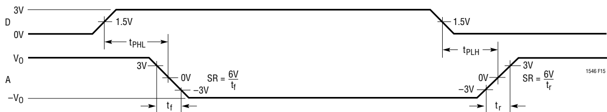
Figure 15. V.28 Driver Propagation Delays
