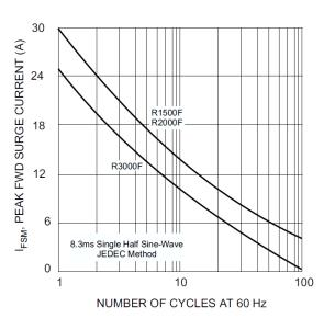
Fig. 3 Peak Fwd Surge Current vs # of Cycles @ 60 Hz
