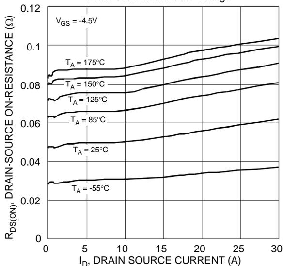
Figure 5 Typical On-Resistance vs. Drain Current and Temperature
