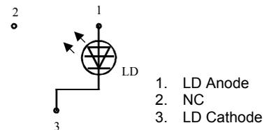
\* This model does not have Photo Diode.
