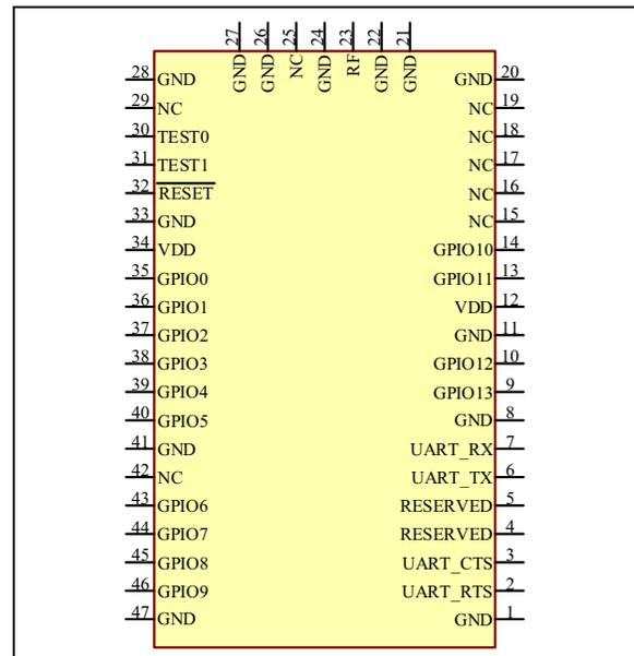
**FIGURE 1-3: RN2903 BLOCK DIAGRAM**
