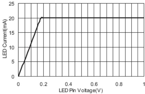
LED Current VS Input Voltage
