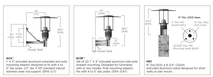
NOTE 1: PCA Pole with ACA attachment requires a 30" (762) tenon extension over pole nominal height. EC3P and EC3PS require an 18" tenon extension. Factory installed.
