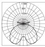
Descriptive Information Total Lms: 4957 Lumens Total Input Watts: 128 W Lamps: ED17/Clear Metal Halide Total efficiency: 55% BUG Rating: B2-U3-G1 Cutoff classification: Semi-Cutoff Distribution: Type V
