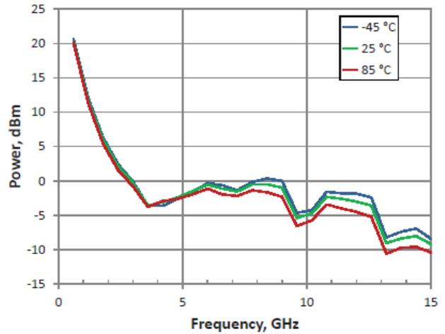
Typical Performance Curves @ 1000 MHz over temperature using SMT580 package:
