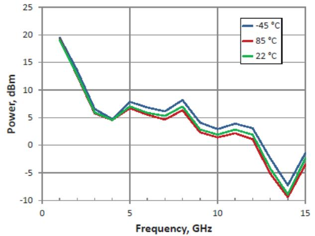
Typical Performance Curves @ 1500 MHz over temperature using SMT580 package:
