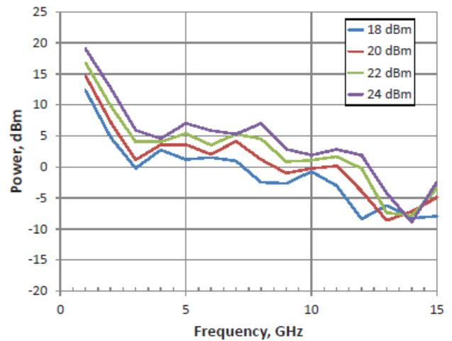
**Harmonic Output, 1500 MHz Input Frequency**
