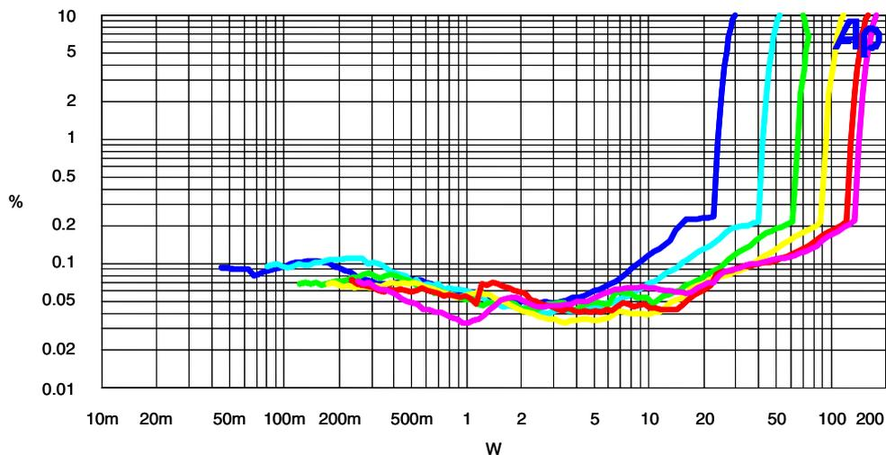
**4.2 THD+Noise Ratio versus Output Power at different input power supply Input frequency: 1KHz; Output load: 2.67Ω;**
