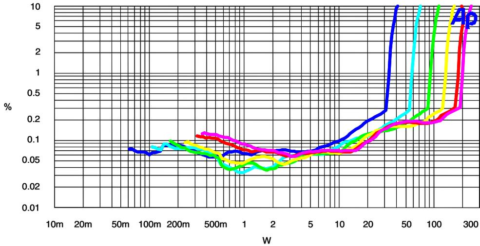
**4.3 THD+Noise Ratio versus Output Power at different input power supply Input frequency: 1KHz; Output load: 2Ω;**
