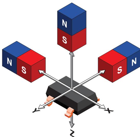
**Figure 1: Three Dimensions of Magnet Orientation.**
