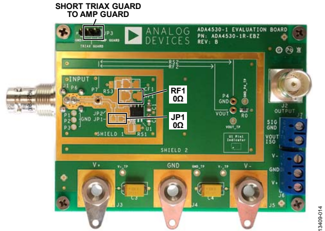
Figure 7. Buffer with Triax Guard Driven by Amp Guard
