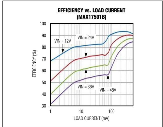
Figure 3. MAX17501B Efficiency
