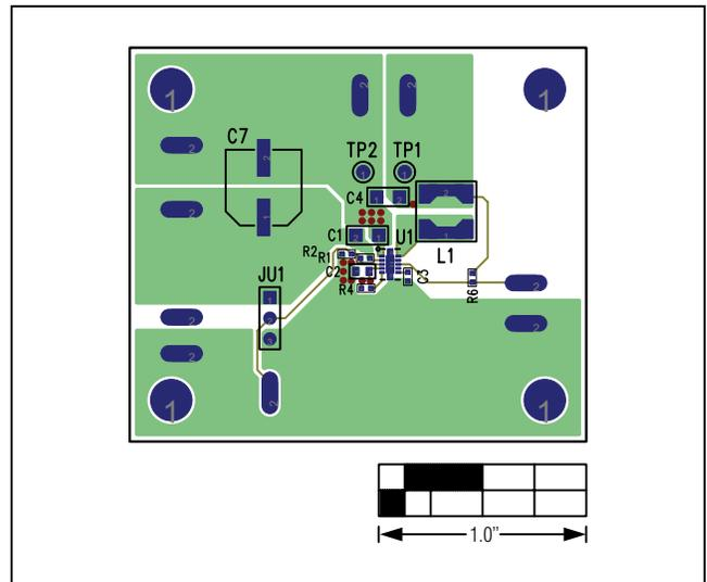
Figure 12. MAX17501B/MAX17501F EV Kits PCB Layout—Component Side
