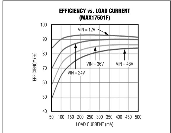
Figure 4. MAX17501F Efficiency
