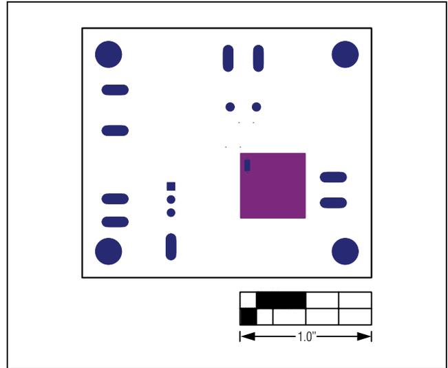
Figure 15. MAX17501B/MAX17501F EV Kits PCB Layout—Bottom Solder Mask
