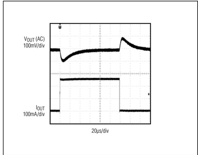
Figure 7. MAX17501F No Load to 250mA Load Transient
