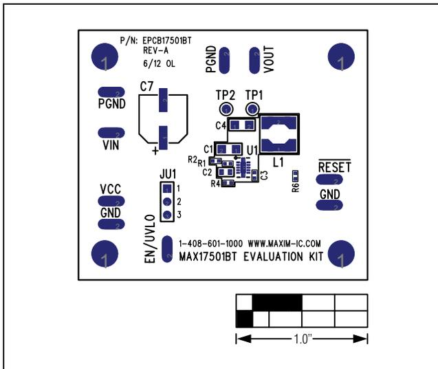
Figure 10. MAX17501B EV Kit Component Placement Guide—Component Side
