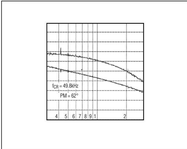
Figure 5. MAX17501B/MAX17501F Full-Load Bode Plot ( $V_{IN} = 24V$ )
