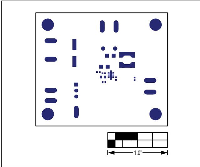
Figure 14. MAX17501B/MAX17501F EV Kits PCB Layout—Top Solder Mask
