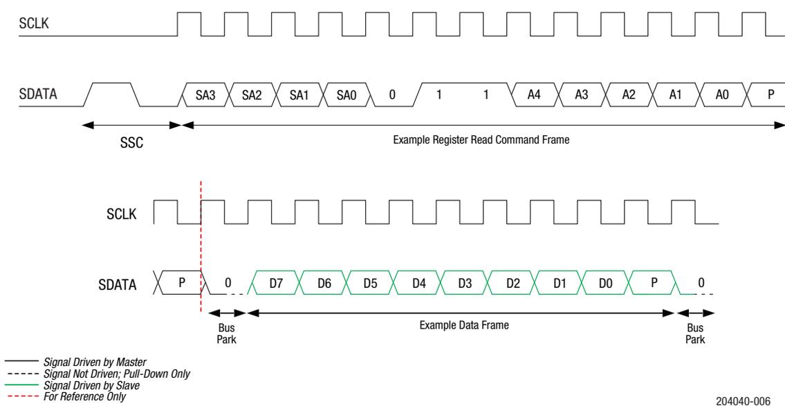
**Figure 6. Register Read Command Timing Diagram**
