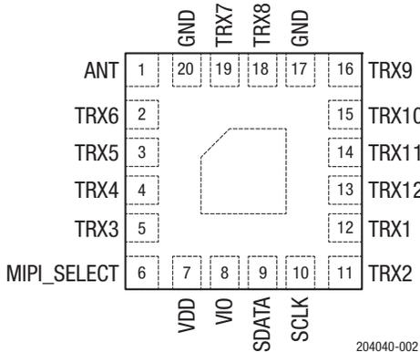
Figure 2. SKYA21052 Pinout (Top View)
