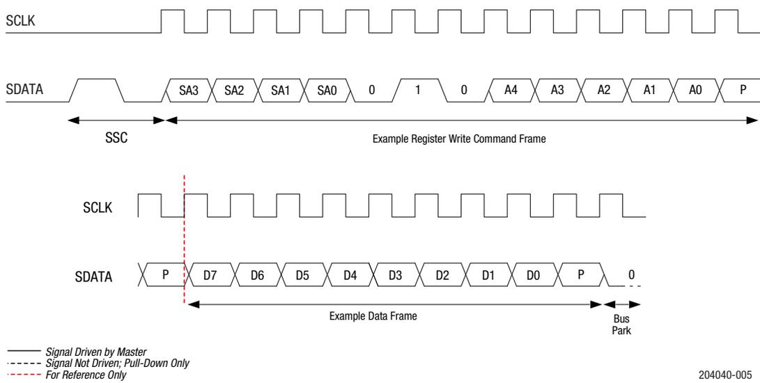
**Figure 5. Register Write Command Timing Diagram**
