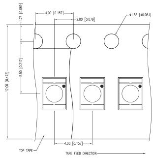
\*UNLESS OTHERWISE SPECIFIED TOLERANCES PER DECIMAL PRECISION ARE: X=±1 (±0.039), X.X=±0.5 (±0.020), X.XX=±0.25 (±0.010), X.XXX=±0.127 (±0.005). LEAD SIZE=±0.05 (±0.002), LEAD LENGTH=±0.75 (±0.030). MIN=  $^{+DECIMAL}_{-0.00}$  PRECISION MAX.=  $^{+0.00}_{-0.00}$  MAX.=  $^{+$
