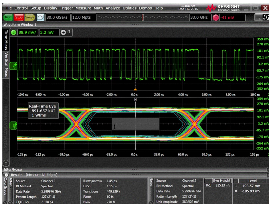
Figure 3. The BER contour is computed statistically from jitter and noise components.
