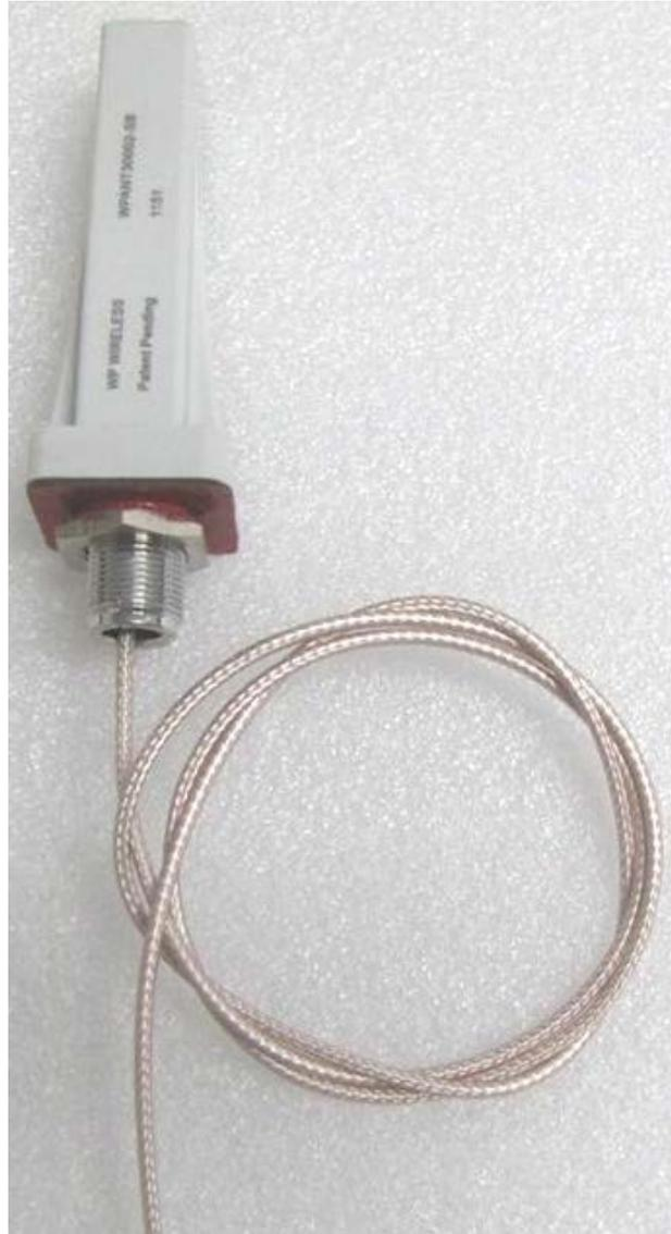
Note: Prototype shown here. The actual antenna will have 10" long cable with straight SMA Male connector.
