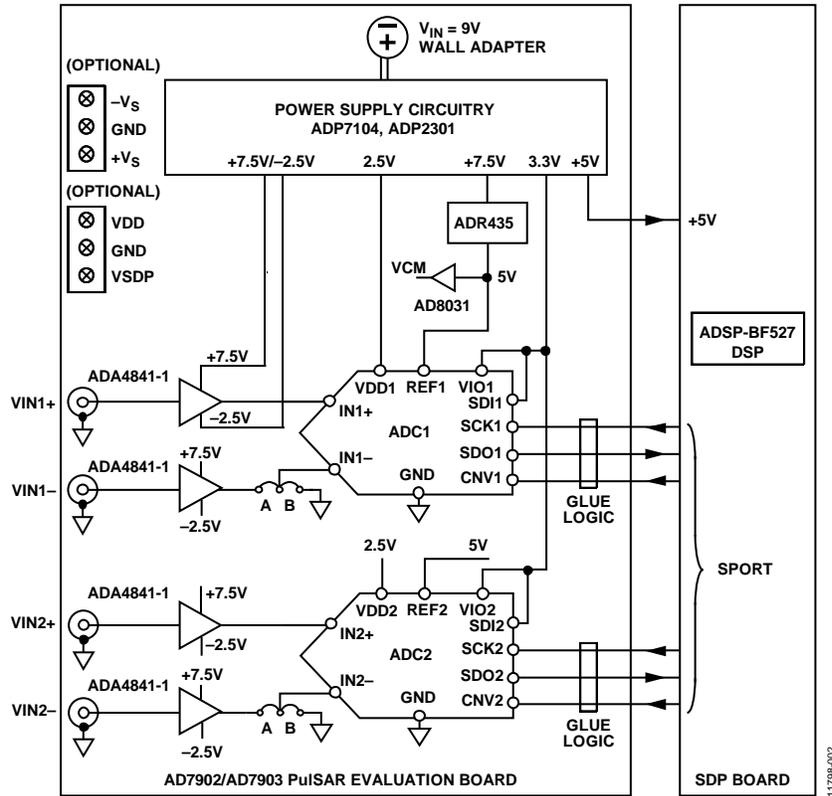
Figure 16. Simplified Evaluation Board Functional Block Diagram
