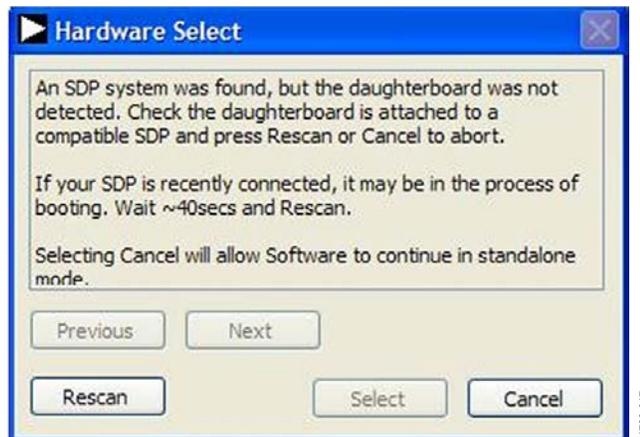
Figure 17. SDP Board Not Connected to the USB Port Pop-Up Window Error
