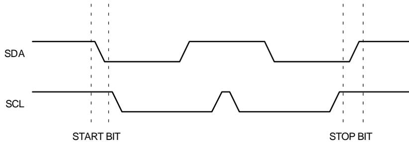
Figure 4. Start/Stop Timing
