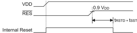
Note:  $t_{RSTD}$  is power-on delay, typical time=50ms
