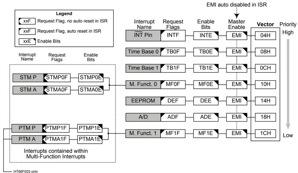
**Interrupt Structure – HT66F002/HT66F0025/HT66F003**
