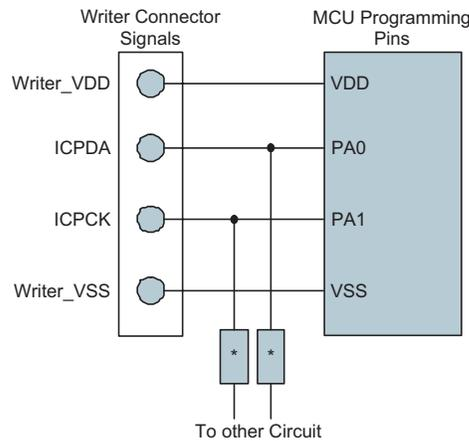
Note: \* may be resistor or capacitor. The resistance of \* must be greater than 1k $\Omega$  or the capacitance of \* must be less than 1nF.
