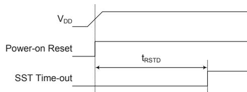
Note:  $t_{RSTD}$  is power-on delay, typical time=50ms
