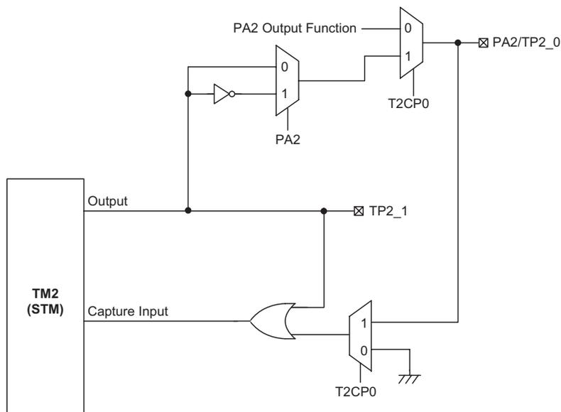
**TM2 Function Pin Control Block Diagram**
