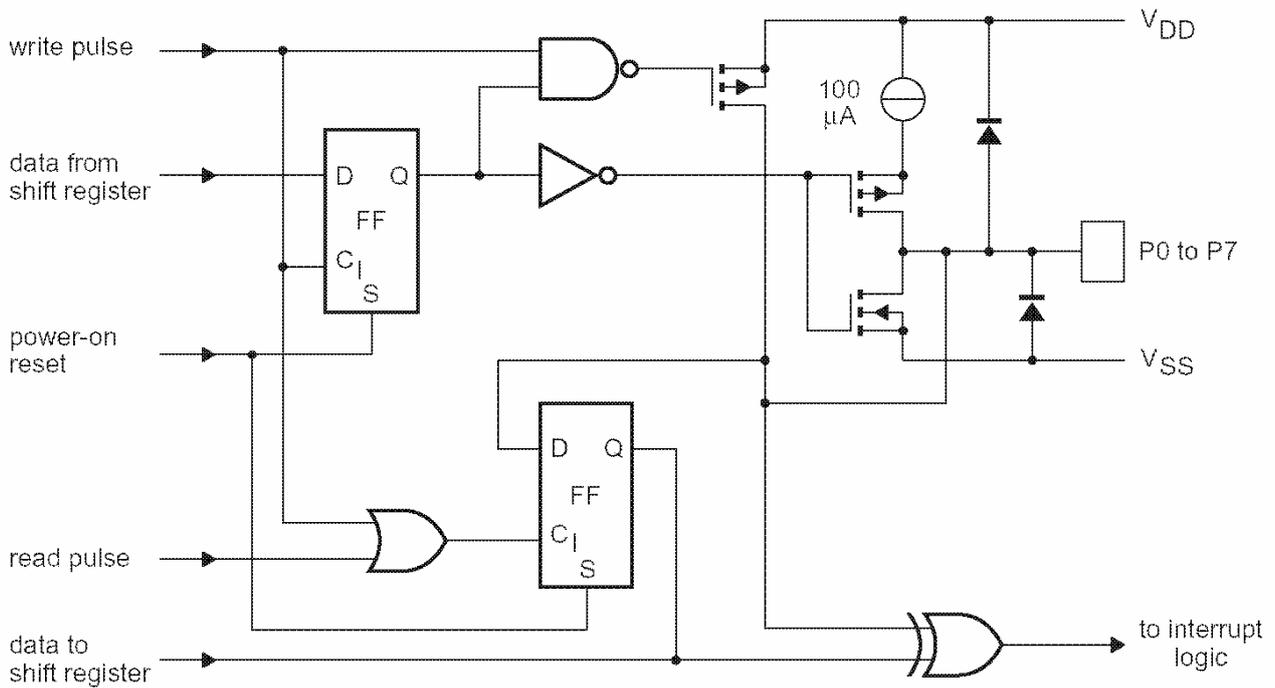
*Simplified schematic diagram of each Port.*
