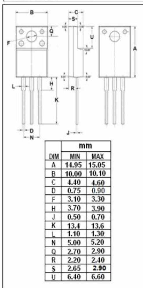
**iscN-Channel MOSFET Transistor****2SK3564, I2SK3564****ELECTRICAL CHARACTERISTICS** $T_c=25^\circ\text{C}$  unless otherwise specified
