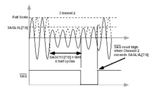
The 12-bit SAGLVL register contains the amplitude that the voltage channel must fall below before sag event occurs. The sag threshold is the number of half line cycles below which the voltage channel must remain before a sag condition occurs. Each LSB of the SAGCYC register corresponds to one half line cycle period. The default value is 0xFF(HEX). At 50Hz, the maximum sag cycle time is 2.55 seconds.
